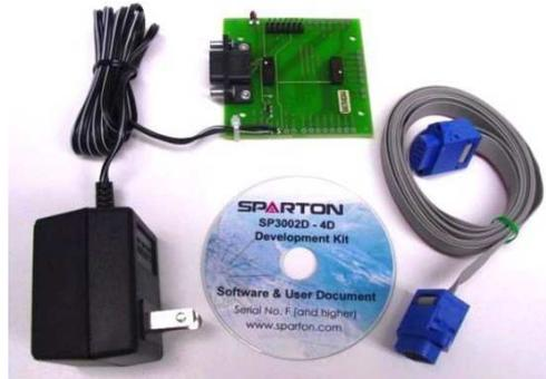
Figura 1.3 SPARTON SP3002D-4D KIT COMPASS DEVELOPMENT KIT
