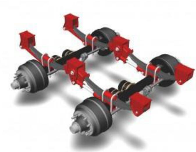
**FIGURA 1.12 SUSPENSION BIAxIAL (PARA DOS EJES) (Ref. 1)**
