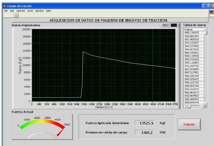
FIGURA 3.7. CURVA FUERZA VS TIEMPO, PROBETA 4 EXTRUIDA
