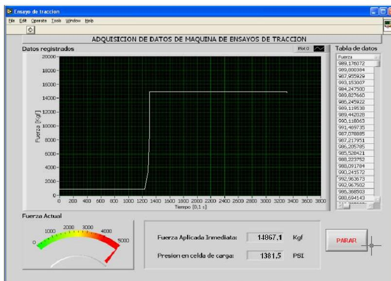
FIGURA 3.5. CURVA FUERZA VS TIEMPO, PROBETA 2 EXTRUIDA
