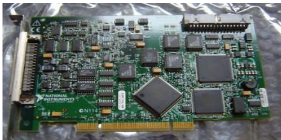
Figura 3.3 DAQ PCI-6024E de National Instruments
