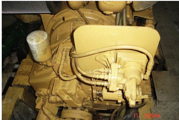
FIGURA 1.11 REDUCTOR ZF – 350 a 2.63:1
