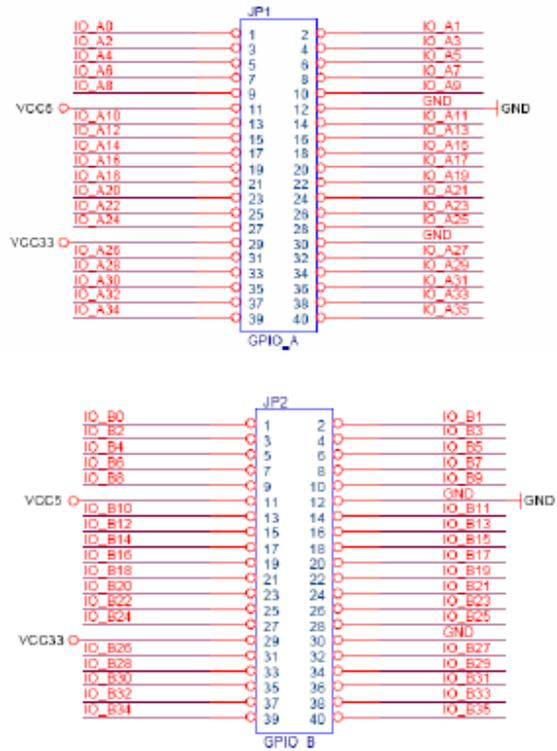
Figure 3.10 Two 40-pin Expansion Headers
