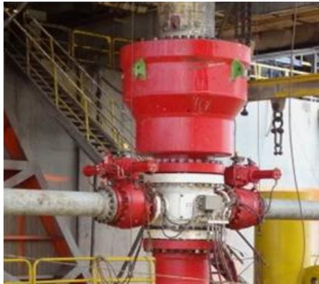
Figura 1.31 Diverter (FUENTE: JVS Engineers, [www.jvsengg.com/pressure-diverter-ball-valve.html](http://www.jvsengg.com/pressure-diverter-ball-valve.html))
