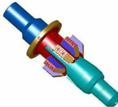
Figura 4.10 Die Collar (FUENTE: <http://www.ingenieriadepetroleo.com/2010/11/herramientas-empleadas-en-la-pesca-de.html>)
