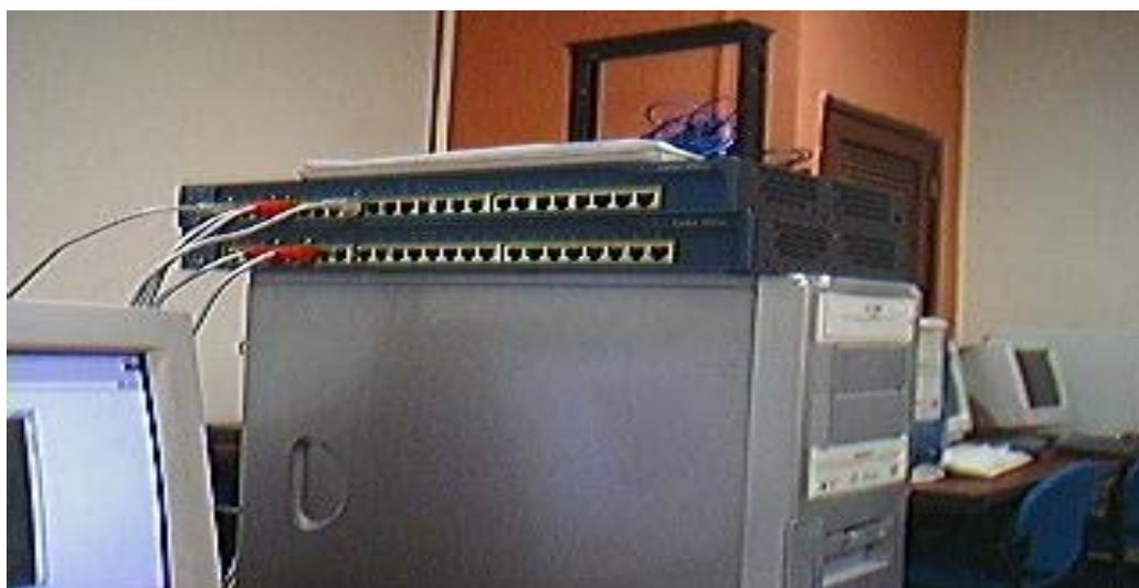
*Figura 4.3 Switch CISCO CATALYST 2950.*
