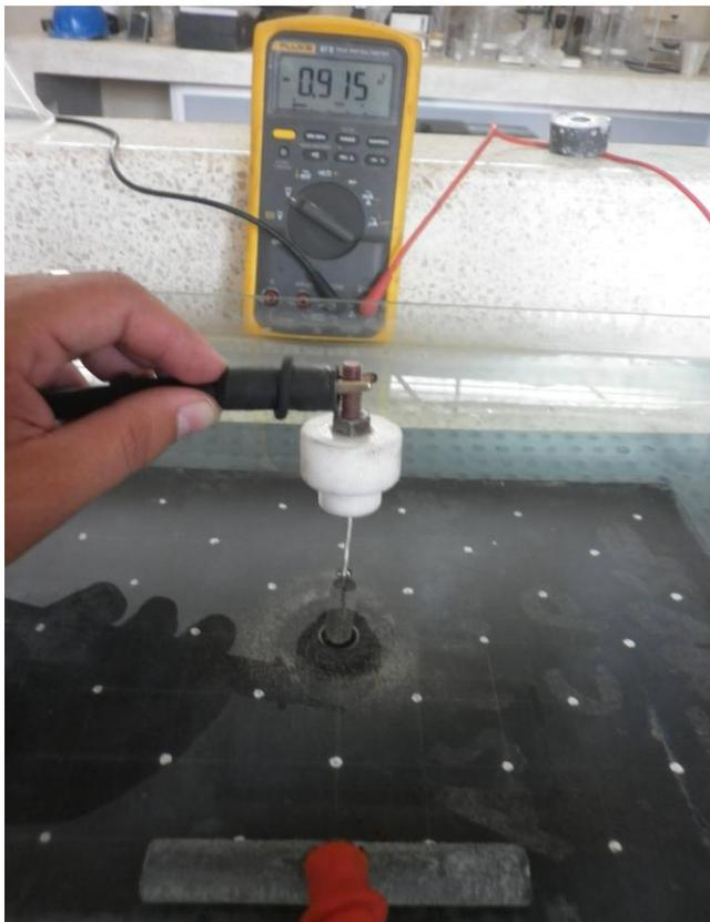
**FIGURA 3.11 POTENCIAL ELECTRODO EXPERIMENTAL.**
