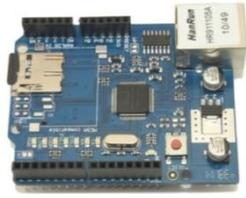
Figura 9. Ethernet Shield W5100.
