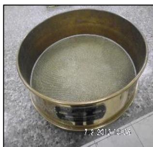
**FIGURA 3.1 USA STANDARD TEST SIEVE**
