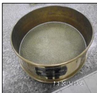
**FIGURA 3.1 USA STANDARD TEST SIEVE**
