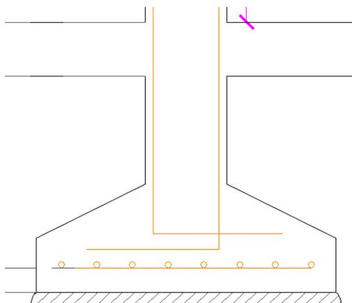
**Figura 3.31: Detalle; zapata-pedestal-riostra.**
