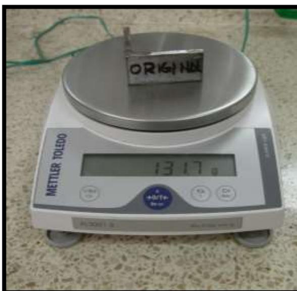
**FIGURA 2.1 PESAJE DE PROBETAS**
