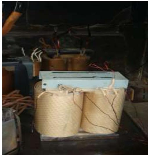
**FIGURA 1.3 BOBINA Y NÚCLEO DE UN TRANSFORMADOR
