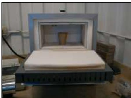
**FIGURA 2.4 HORNO ELÉCTRICO CON CRISOL DENTRO.**
