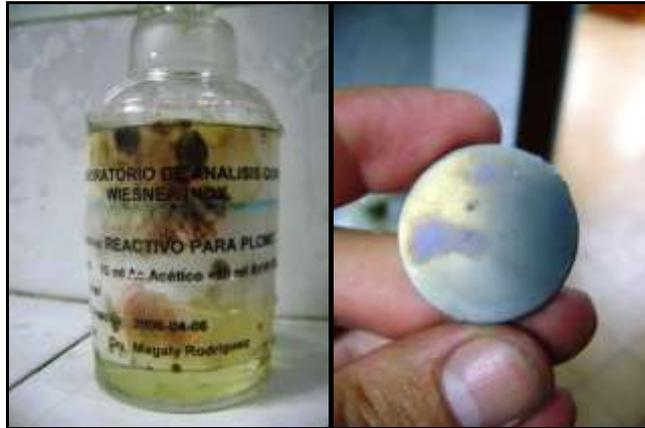
**FIGURA 2.15 REACTIVO QUÍMICO Y PROBETA “ATACADA”**
