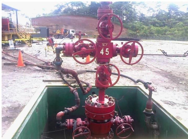
**FIGURA 2.14: Cabezal**
