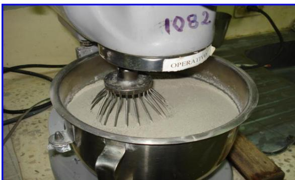
**FIGURA 3.16. HOMOGENIZANDO CEMENTO + ZEOLITA**
