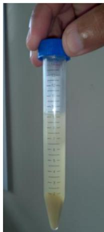
**FIGURA 4.74 RESINA EPÓXICA GE-60 + NANOARCILLA NA MINUTO 30.**
