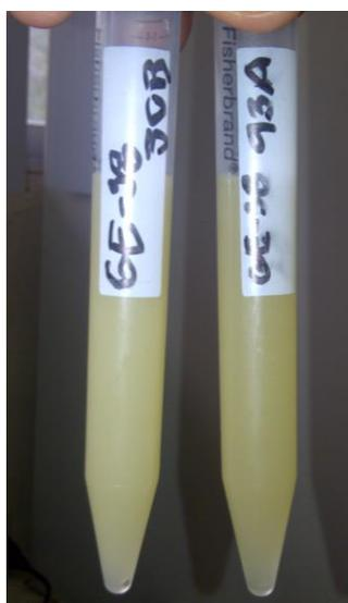
**FIGURA 4.105 RESINA EPÓXICA GE-38 + NANOARCILLA 30B,
