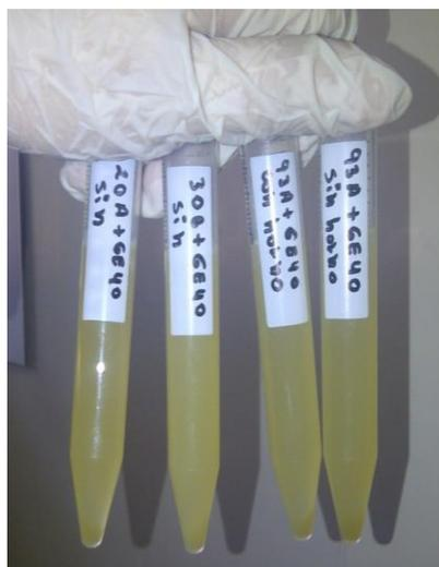
**FIGURA 4.90 RESINA EPÓXICA GE-40 + NANOARCILLA 20A, 30B, 93A CON HORNO Y SIN HORNO MINUTO 30**
