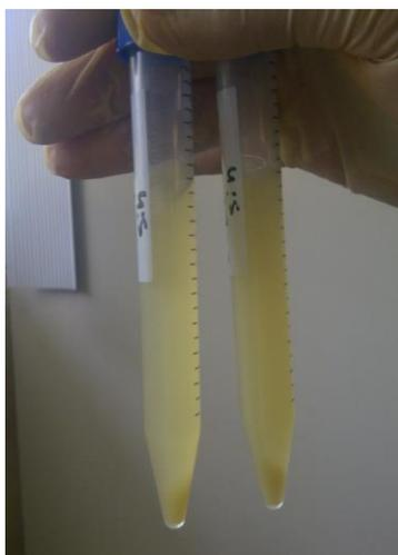
**FIGURA 4.78 RESINA EPÓXICA GE-38 + NANOARCILLA
