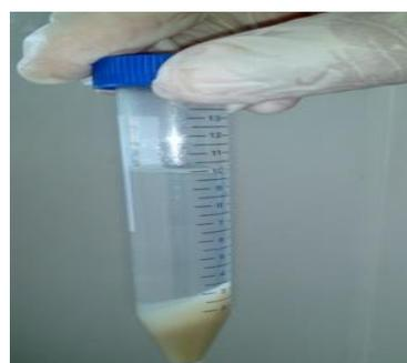
**FIGURA 4.16 AMINA D-230 + NANOARCILLA NA +
