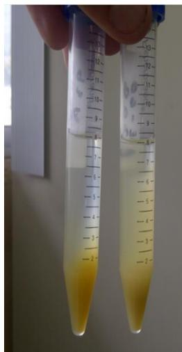
**FIGURA 4.104 RESINA EPÓXICA GE-60 + NANOARCILLA 30B,
