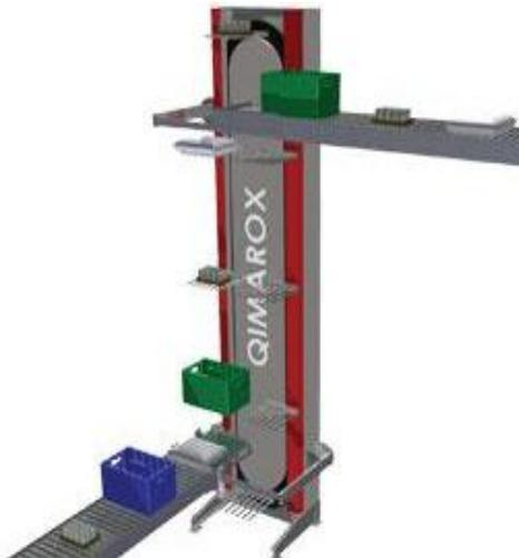
**Figura 1.2 Transportador Vertical Continuo**
