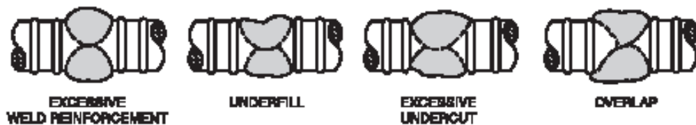
(E) UNACCEPTABLE GROOVE WELD PROFILES IN BUTT JOINTS
