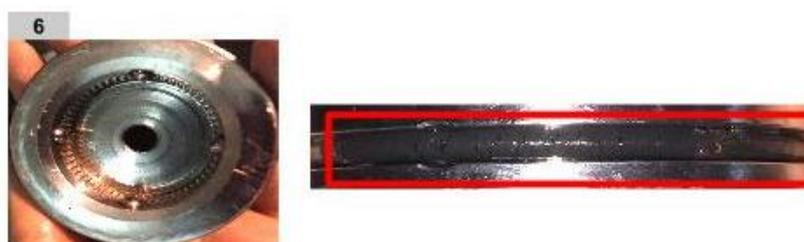
**Figura A.44: Chuck y O-ring # 6.**
