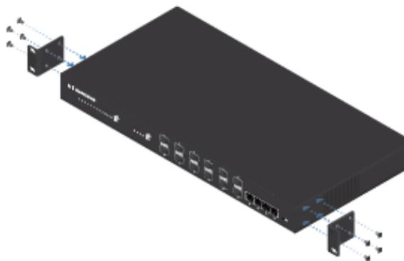
Attaching Rack-Mount Brackets to the EdgeSwitch XG
