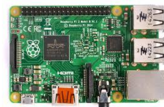
Figura 2.6: Vista superior de la Raspberry Pi 2 Model B
