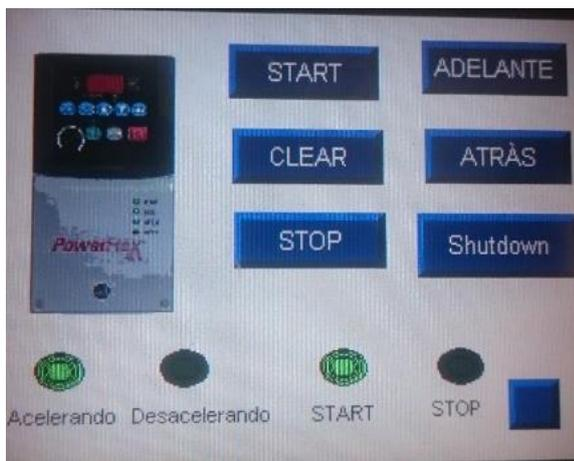
**Figura 55: Modo “Forward” del HMI**
