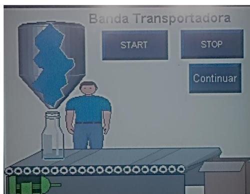
Figura 32: Panel View Plus 600 presionando “START”
