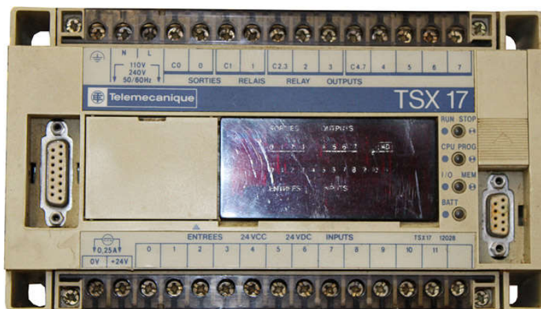
Figura 6. PLC Telemecanique TSX17
