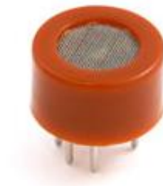
Figura 2.4.2 – Sensor de Gas MQ3 [6]
