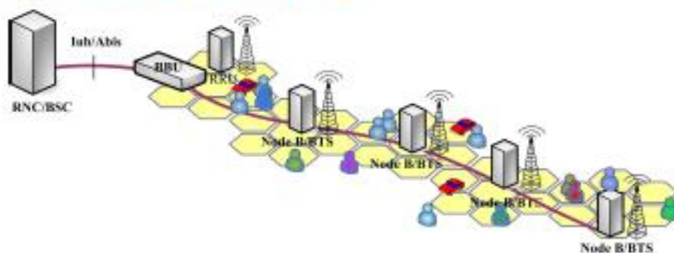
FIGURE 8 CHAIN NETWORKING AT ABIS INTERFACE
