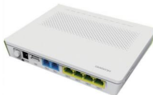
Figura 3.11: Optical Network Terminal (ONT) HG8245 [6]
