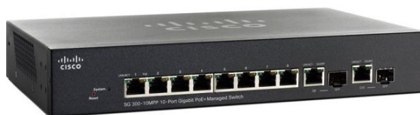
Figura 3.11 Switch Cisco SG300
