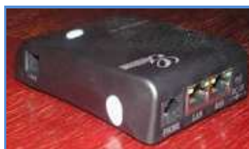
Figura 1.8 Analog Telephony Adapter VoIP Grandstream HT486
