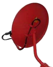
Figura 4.16 Lazo de cable coaxial [36]
