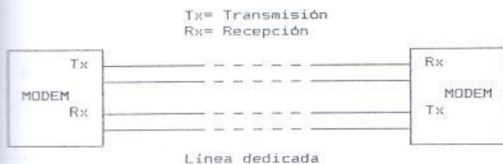
Fig. 4.3. CIRCUITO SIN DIAL BACK-UP.
