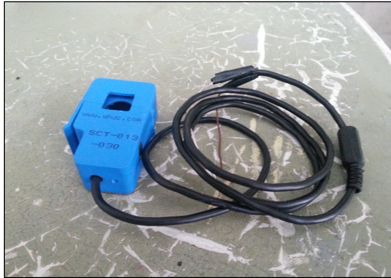
Figura 2.11. Non-invasive AC current sensor
