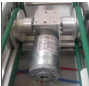
Figura 2.5: Motor reductor DC
