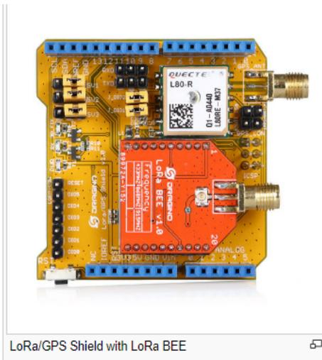
LoRa/GPS Shield with LoRa BEE
