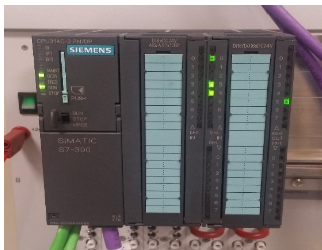
Figura 2.12: PLC SIEMENS SIMATIC S7-300.
