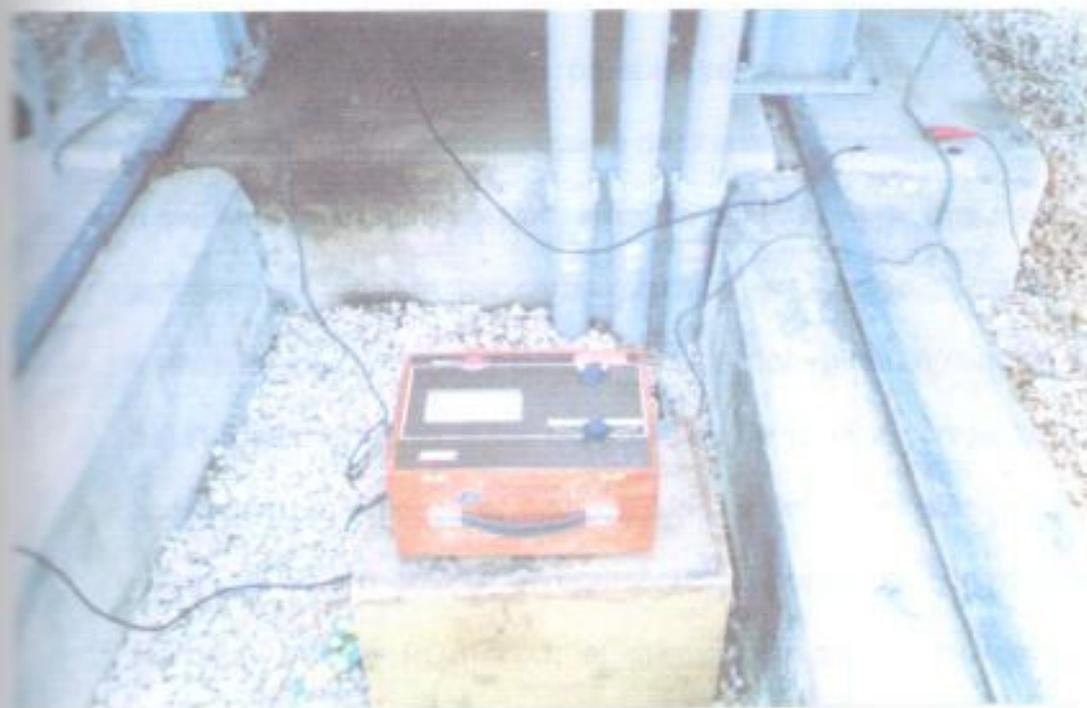
**FIG. 3.5 Megger BIDDLE 5000 VDC (motorizado 120 VAC)**
