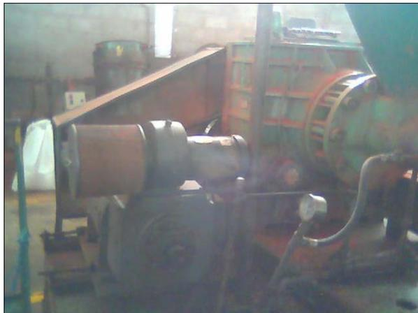
**Fig. 1.2 Vista Real Motor Extrusor**
