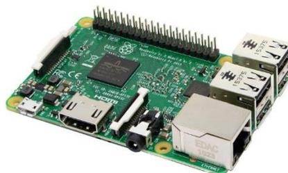
**Figura 3.2: Raspberry Pi 2 Modelo B**
