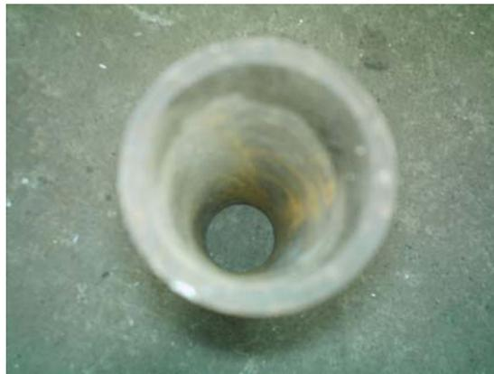
**FIGURA 3.6. TUBERÍA DESPUÉS DE LA LIMPIEZA QUÍMICA.**
