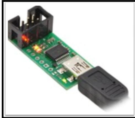
Figura 2.9 Pololu USB AVR Programmer
