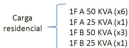
$$I_n = \frac{50 \text{ KVA}}{7,62 \text{ KV}} = 6,56 \text{ Amp.} \quad I_n = \frac{25 \text{ KVA}}{7,62 \text{ KV}} = 3,28 \text{ Amp.}$$
