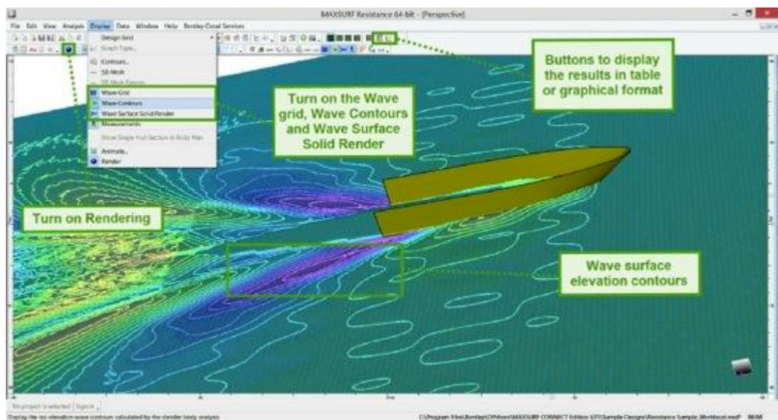
Following, Figures 84 to 87 shows the wave surface elevation contours for demi and twin hulls at  $F_n=0.34$  in two Load Conditions.
