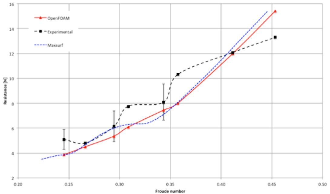
**Figure 71:** Total resistance of catamaran hull at different Froude number – Full Condition
