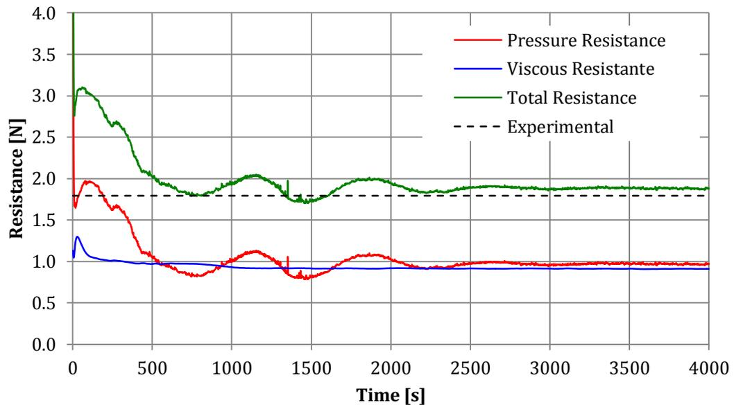
Total resistance was obtained by adding pressure and viscous forces.
