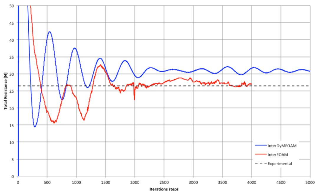
**Figure 49:** Total resistance over the time with different solvers at  $Fn=0.218$
