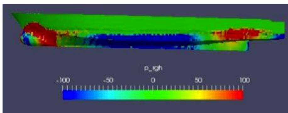
**Figure 75:** OUTSIDE Twin hull dynamic pressure around the hull at  $F_n=0.34$
