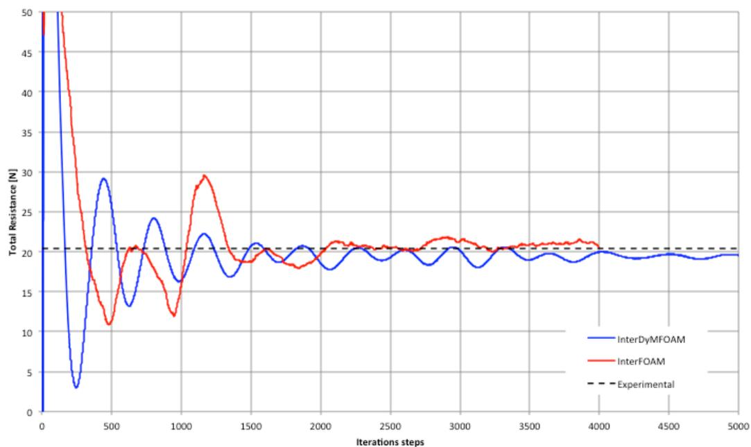
**Figure 46:** Total resistance over the time with different solvers at  $Fn=0.183$
