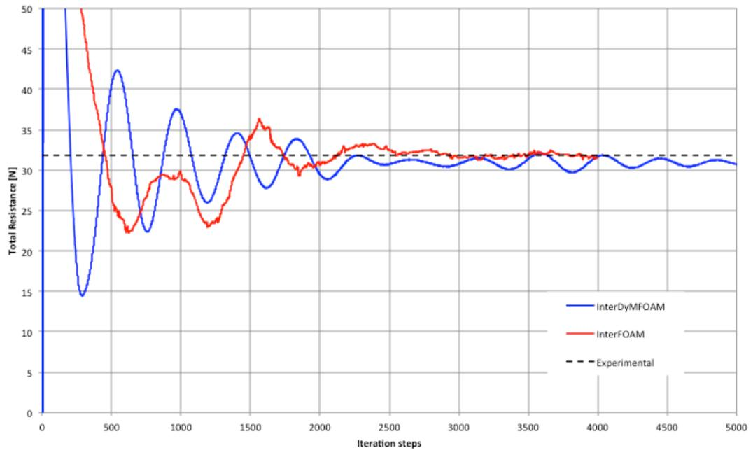
To compare with the experimental results, DTC Hull case was run at different Froude numbers. Table 18 shows the results of model test and numerical simulation using interFoam, as static method, and interDyMFOAM, as a dynamic method.
