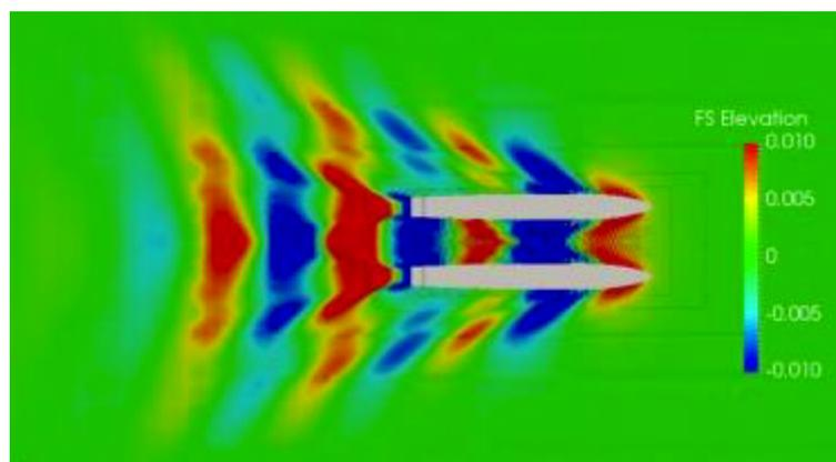
**Figure 81:** Wave pattern at  $Fn=0.34$
