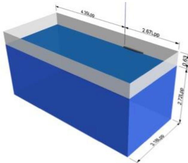
In the first step, BlockMeshDict file creates a background mesh with blocks using vertices (points). For example, the following block is defined as hexagonal with 42, 19 and 50 cells in the x, y, and z direction respectively. Finally a simpleGrading expansion type and its ratio are reviewed.
