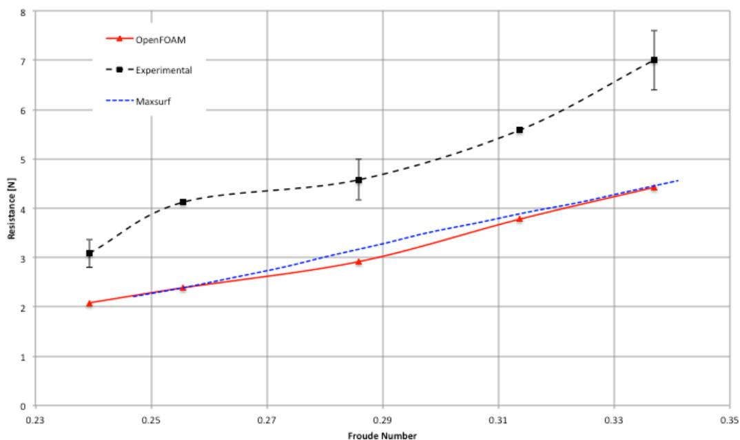
**Table 24:** Total resistance components for Demi hull
