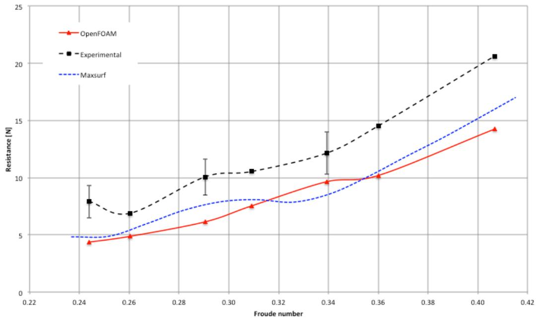
The errors between experimental data and numerical simulations are lower in light condition of catamaran. However none of the curves follows the same trend.
