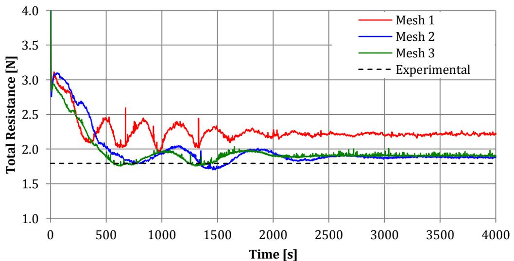
Four thousand values of resistance were generated at the Light Load condition at  $v=1.05$  [m/s]. Table 21 shows the average of the last five hundred values for the resistance of each mesh and its error when compared with an experimental value of  $R_{t\text{ exp}}=1.79$  [N].
