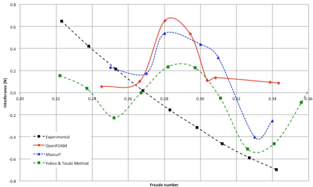
The interference factor obtained by numerical simulations is linear contrasting with the experimental interference published by Chávez and Lucín [1]. The positive interference corresponds to increased interference (unfavorable) and the negative values to decrease (favorable).
