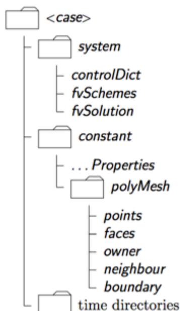
Figure 11 contains the standard set of keyboard entries of all data file of OpenFOAM. This entry provides a brief description of the each file, as: the format version, the data format (ascii or binary), the class of data file (typically *dictionary*) and the object or file name.
