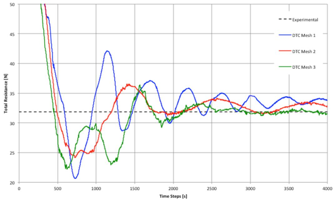
**Table 17:** Numerical Resistance Error for different Meshes
