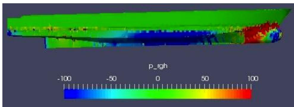
Bolbuos is the zone with greater pressure; Figure 76 shows the pressure in this zone, outside the hull.
