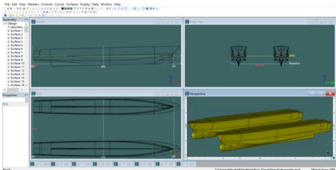
Maxsurf Resistance module it's a wave and power prediction tool. Use a range of industry standard algorithms, allowing the user to select the method to implement. The calculations methods that provided Maxsurf for resistance are: Savitsky pre-planning and planning; Lahtiharju for planning vessels;
