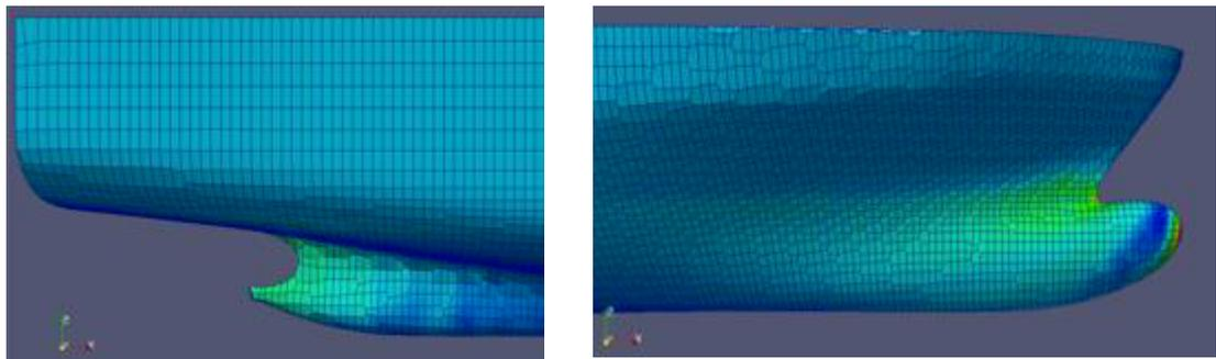
To capture the free surface interface, air and water, the volume of fluid (VoF) algorithm is used. This requires additional refinement on 3 and 4 zones. Toposet files create boxes around the hull and generate other zones of refinement. Figures 19 and 20 shows six boxes created by Toposet files.
