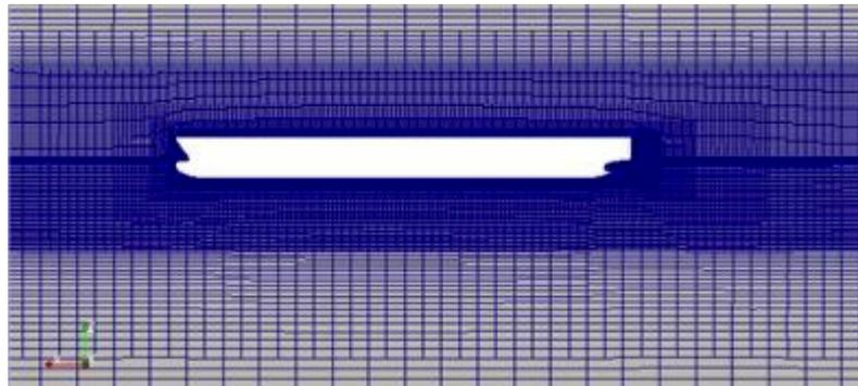
The value of  $y^+$  is used as a way to visualize the distribution of cells around the hull and check the quality of the mesh that captures the boundary layer developed. The range of  $y^+$  has to be  $30 < y^+ < 100$  [11]. Figures 33 to 35 show the  $y^+$  distribution around the DTC Hull for three different meshes after 4000 iterations.  $y^+$  was calculated only for one fluid, fresh water, for this reason only the wetted area is considering as reliable.
