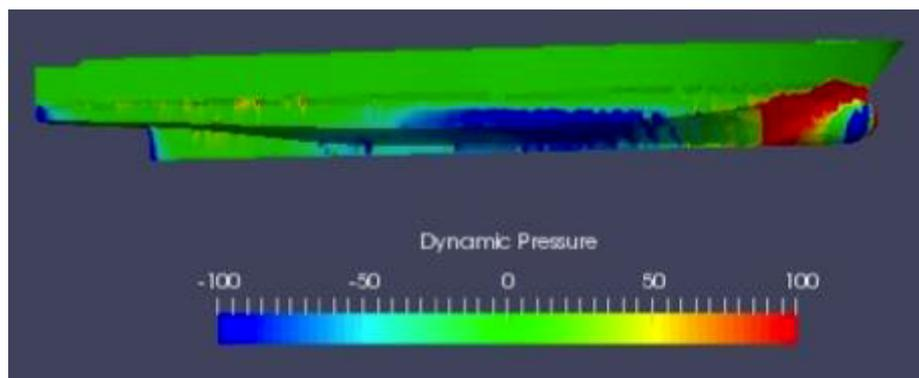
**Figure 74:** INSIDE Twin hull dynamic pressure around the hull at  $F_n=0.34$
