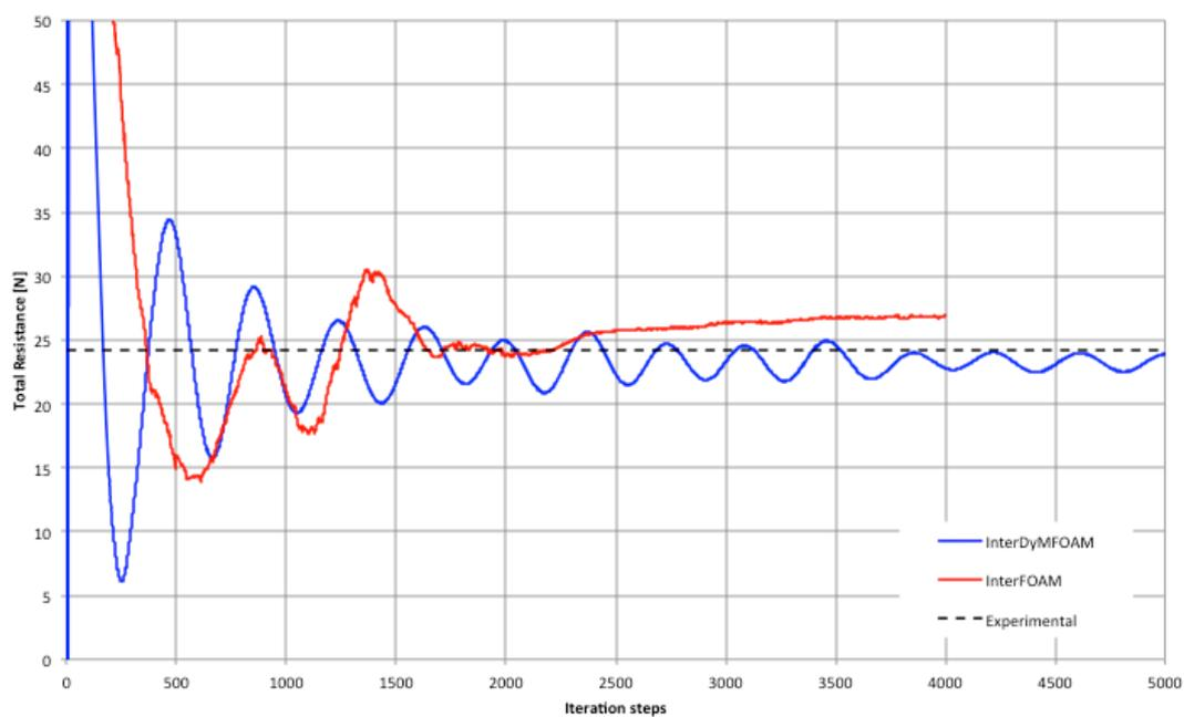
**Figure 48:** Total resistance over the time with different solvers at  $Fn=0.200$
