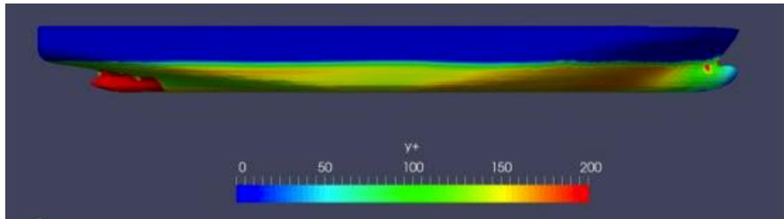
**Figure 34:**  $y^+$  for DTCMesh2 at time 4000 [s]
