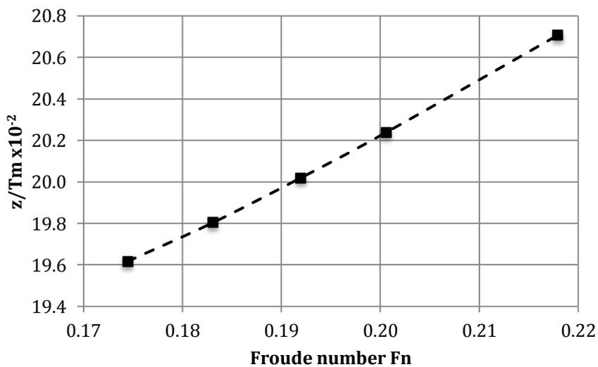
Figure 52 shows the trimming angle at different Froude numbers, the free longitudinal rotation.
