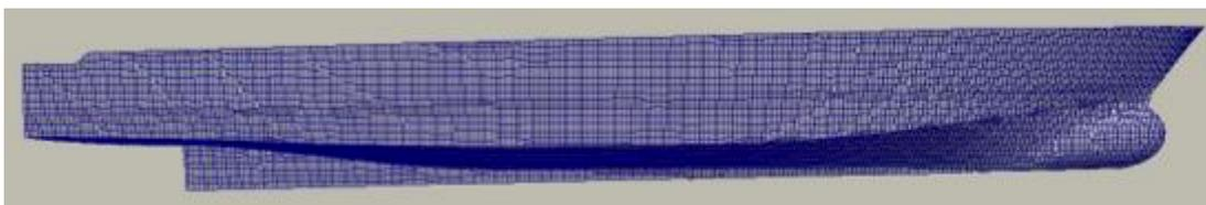
**Figure 58:** Y Plane Mesh 2 Projection
