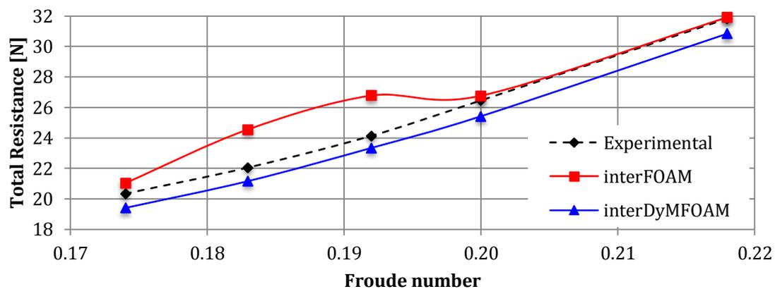
InterDyMFOAM results are closer to experimental data, maybe because the model allowed sinking and trimming in the experiments; the same configuration did it by interDyMFOAM.
