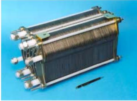
Fig. 3: 100 cell, water cooled, 200 cm 2 active area PEFC stack. Gross dry weight 19.5 kg, volume 14 l.
