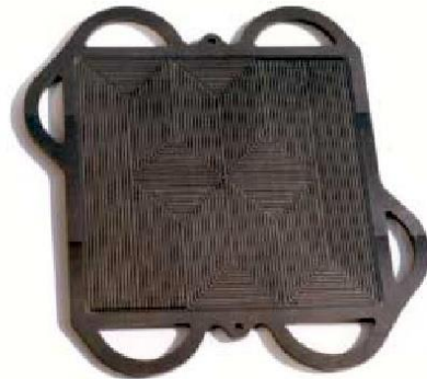
Fig. 2: Bipolar plate with an active area of 200 cm 2 and internal water cooling, as shown schematically in Figure 1.
