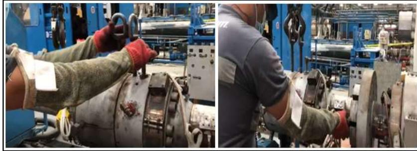
**FIGURA 2.8 AFLOJAR PERNOS DEL ADAPTADOR Y BRIDA PRINCIPAL**
