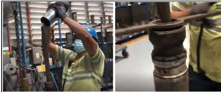
**FIGURA 2.21 ACOPLA DE BOQUILLA CON MACHO DEL MOLDE**
