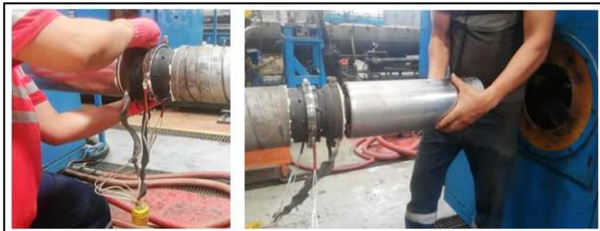
**FIGURA 2.5 DESMONTAJE DE MANDRIL DEL MOLDE**
