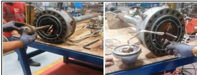
**FIGURA 2.15 ACOPLA DE FLAUTA Y DISTRIBUIDOR DEL MOLDE**
