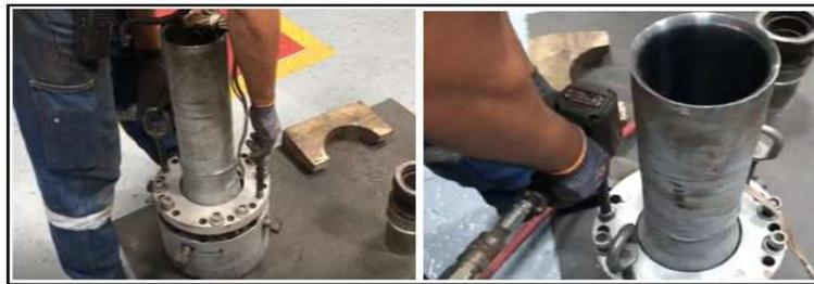
**FIGURA 2.18 ACOPLA HEMBRA FINAL CON BRIDA DEL MOLDE**
