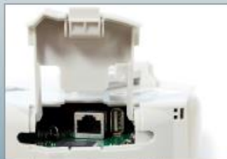
Easy to access enclosure, door latches open
