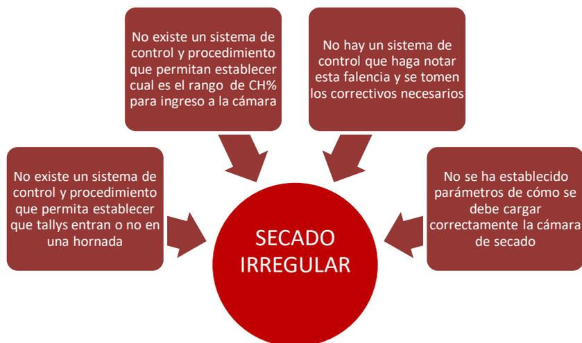
FIGURA 3.15 CAUSAS RAÍZ DEL SECADO IRREGULAR
