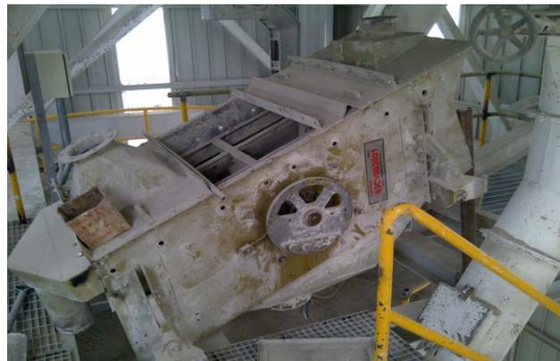
**FIGURA 5.9 - EQUIPO VIBRATORIO CRIBA PRE- INSTALADA**
