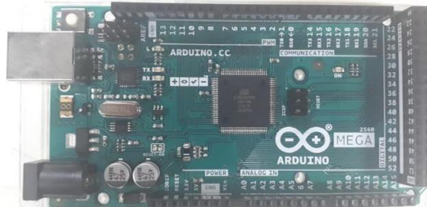
Figura 1.7 Arduino Mega 2560.[7]
